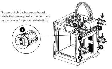
1. Load filaments following the direction shown below.
