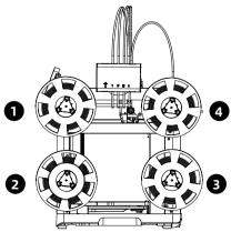
Note: The device can only print if the filament type of the sliced file matches the configured (actually loaded) filament type.
